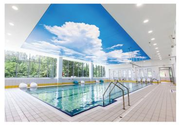
Velaria Systems stretch membranes are waterproof, making them the ideal ceiling system for pool areas or anywhere there are increased levels of moisture or humidity. Instead of absorbing water vapor which could lead damage or mold, water condenses on the surface of the membrane, where it can safely evaporate.
